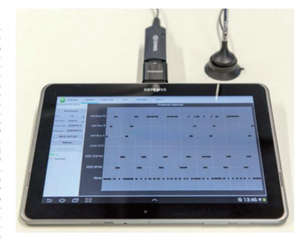
simple and user-friendly tool will be completely sufficient. Fraunhofer IIS has developed an easy to use Android app that uses a DVB-T receiver to analyze the license-free 868 MHz frequency band. Different standards can be recognized locally and without specific knowledge.
